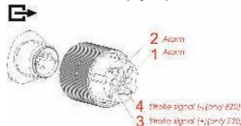
Fig. 12.7 Connector for empty report, fault and stroke signal output:
